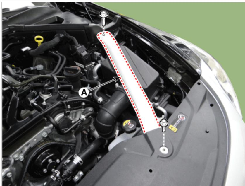
3. Remove the reservoir tank (A).
